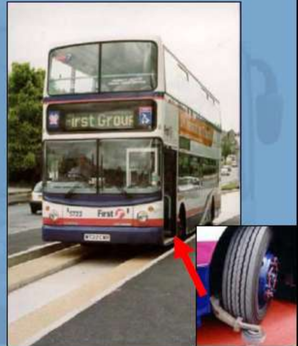
Guided busway (Leeds, London)
