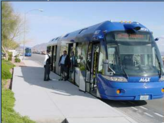
MAX BRT vehicle with multi-door level boarding (Las Vegas, NV)
