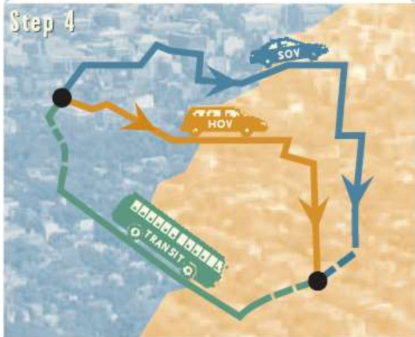
Trip assignment between two fictitious traffic analysis zones: Selecting the fastest route between zones.
