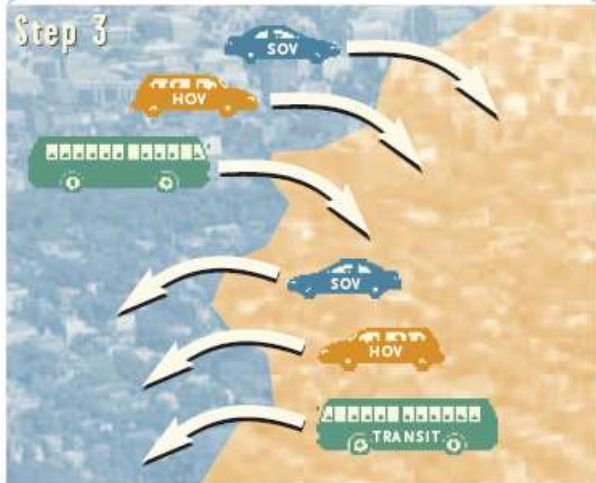
Mode choice between two fictitious traffic analysis zones: Estimating the way people get from zone to zone.
