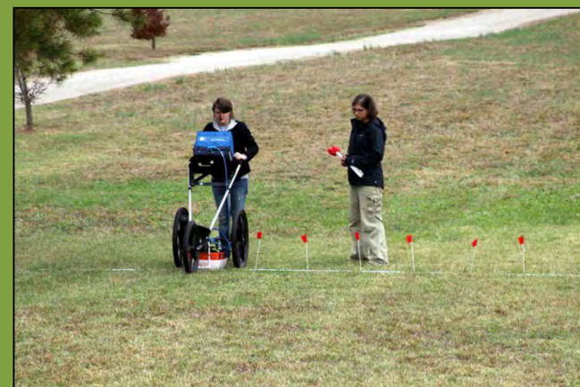
Ground Penetrating Radar Survey of an unmarked cemetery.
