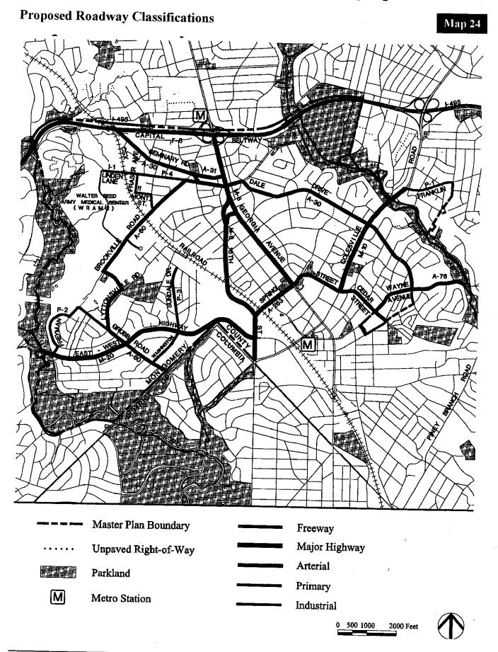
The width of a road's right-of-way helps define its character and ultimate number of lanes. Designating rights-of-way in a master plan reserves land needed for road improvements to accommodate future development. Most of the rights-of-way for North and West Silver Spring roads are unchanged from the previous master plans. (See Table 2.)
