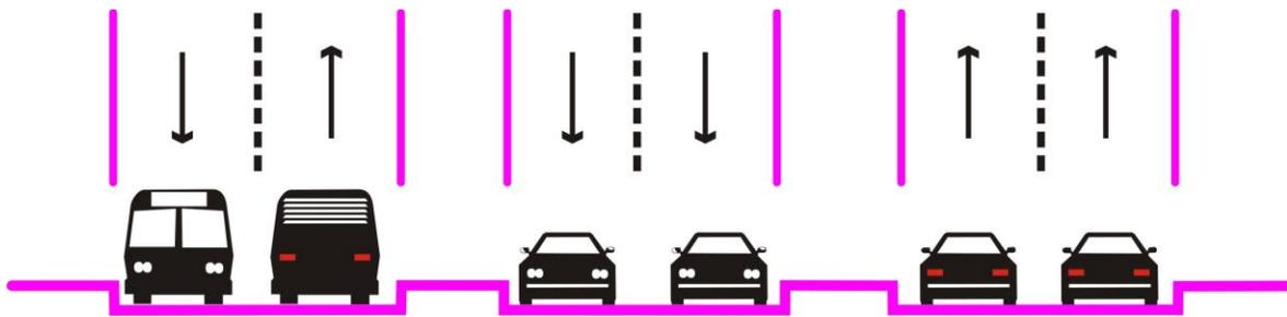
Figure 5 Recommended Corridor Segment Treatment: One-Lane Median Busway
