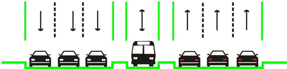
Figure 6 Recommended Corridor Segment Treatment: Managed Lanes
