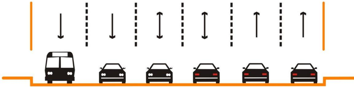
Figure 7 Recommended Corridor Segment Treatment: Curb Lanes
