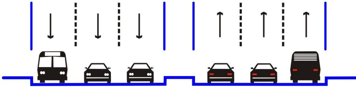
Figure 8 Recommended Corridor Segment Treatment: Mixed Traffic
