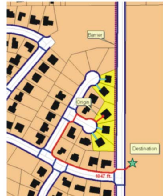
Figure A-3c 1,047 ft. is very accurate, and the barrier is not crossed.
