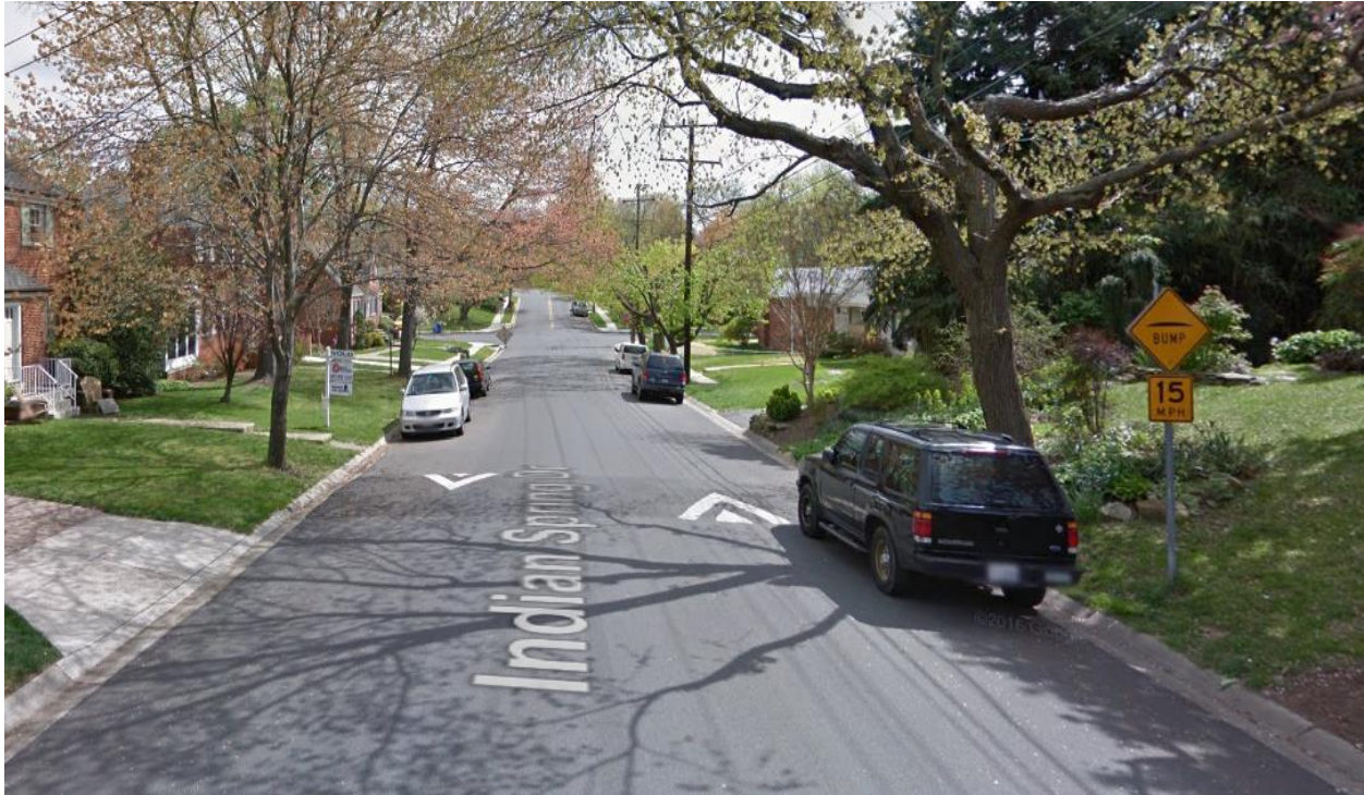
Un-laned, two-way “yield” streets, such as Indian Spring Drive, are common in residential neighborhoods in Montgomery County
