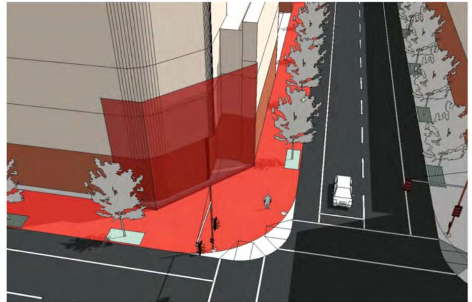
(1) Diagram illustrates corner truncation requirements per 50.26(3) and MCDOT
