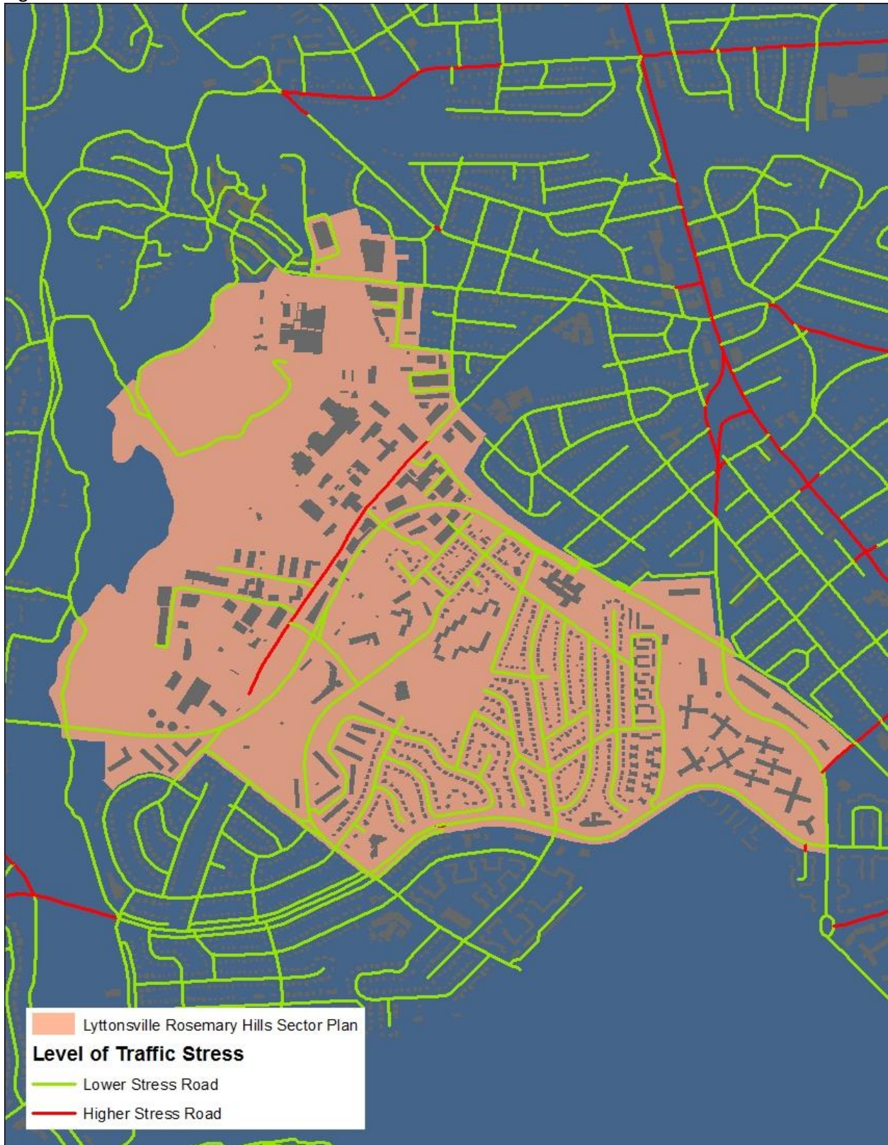
Figure 17: Future Level of Traffic Stress
