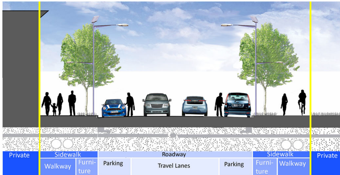
Illustration 17 Gilbert Street Extended Cross Section
