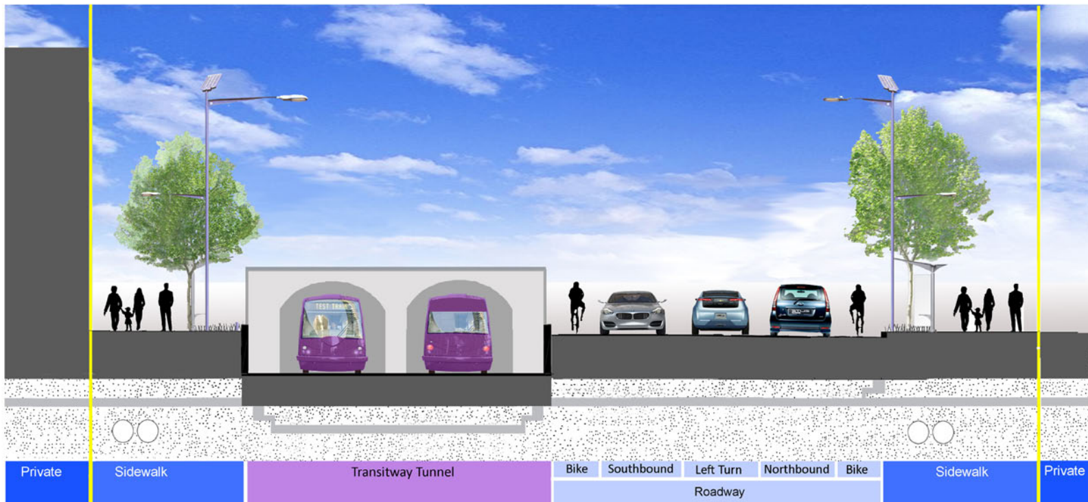
Illustration 5 Arliss Street Cross Section at Tunnel
