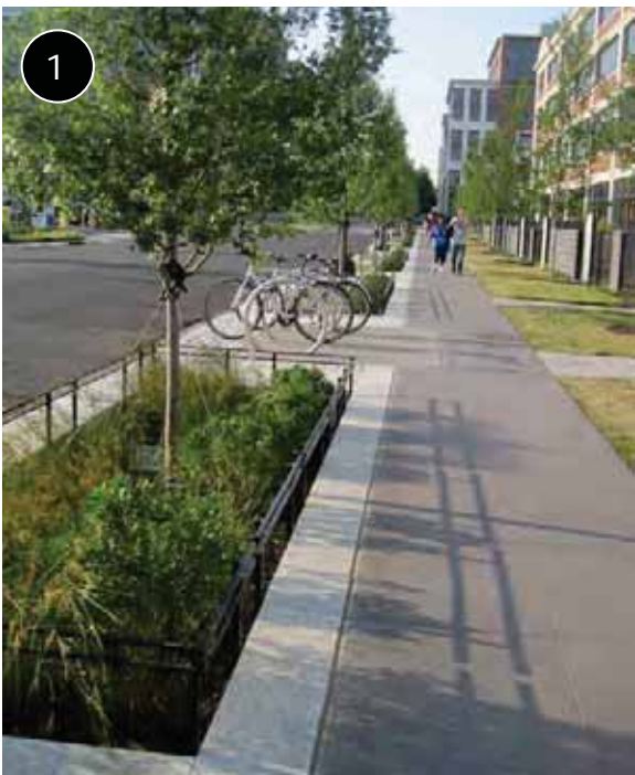
Bioretention in tree boxes
