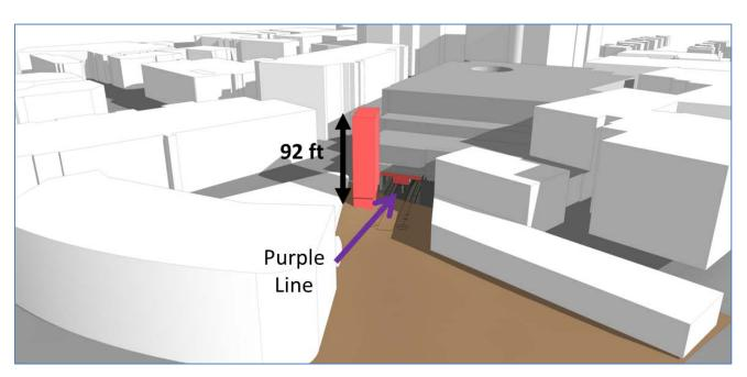
With only a minimum amount of space in the existing tunnel for the Purple Line station, the new south entrance to the Red Line Metrorail station must be located underneath Elm Street, within the public right-of-way. This location negatively impacts the quality of service of the station as follows:
