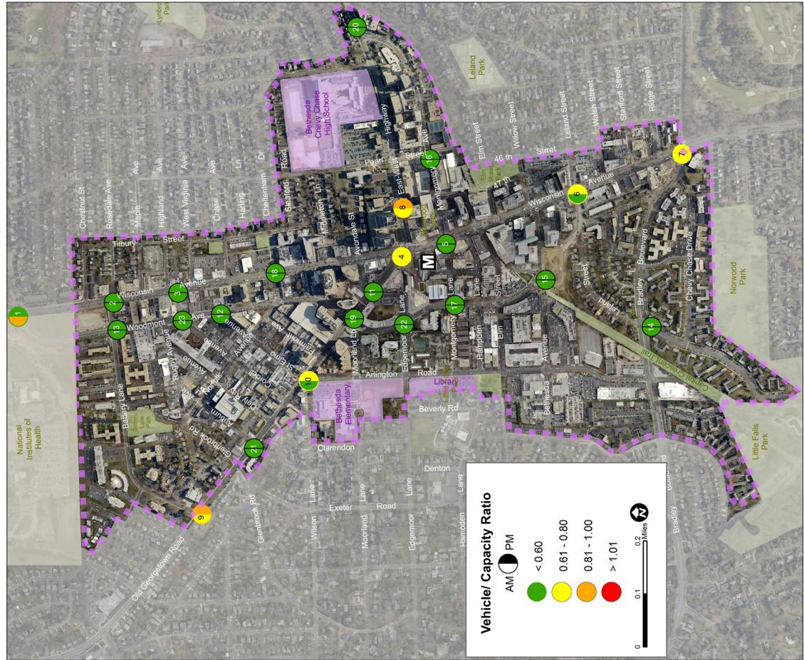
This map illustrates the Vehicle-to-Capacity (V/C) Ratio for Downtown Intersections studied within the last three years (2011-2013). The V/C Ratio provides a measure of traffic congestion that ranges from "No Congestion" (0.00) to "Saturation" (1.00). No Downtown intersections are overburdened by traffic and all are within the policy area congestion standard
